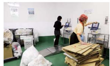
Introduction of a measuring system that collates data on waste amounts by item and feeds the information back to specialty store tenants.
