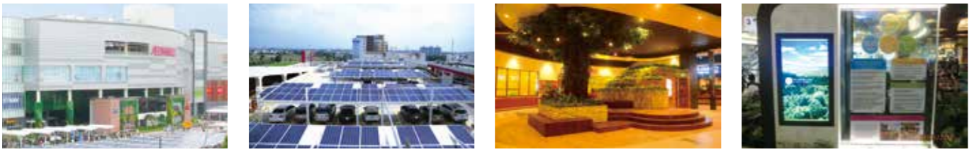
▲ Out mall with a beer restaurant having expansive terrace seats as an anchor tenant. The environment and scenery are given consideration by arranging greenery on and around walls and pillars. ▲ Solar cell modules with a total generating capacity of 320 kWh are installed on the roofs of the parking lot and the motorbike parking space. Our goal is to reduce CO 2 emission by about 270 tons a year. ▲ A forest park designed in the image of a forest is in the restaurant zone on the 3rd floor. Providing a comfortable space where customers can always feel the greenery nearby. ▲ The operating state of the solar power generation facility and various environmental initiatives are introduced to customers at Eco-information.
